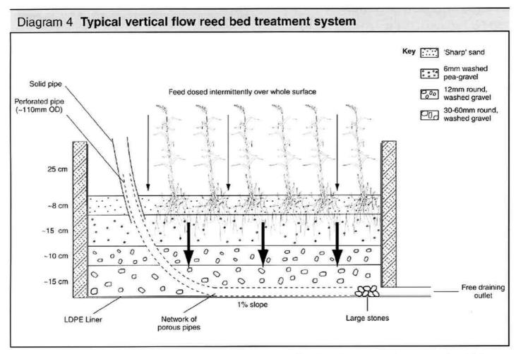
1m to 2m. Vertical flow systems can achieve much better oxygen transfer than horizontal flow systems and therefore achieve more complete treatment, particularly of ammonia. They generally require more maintenance than horizontal systems.
